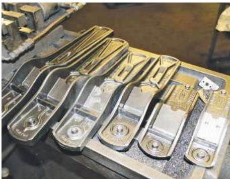
▲ The castings and the subsequent paint job on all the bench planes are done off-site prior to machining
